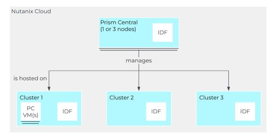
When enabling Prism Central Backup & Restore, the IDF data from Prism Central gets periodically synced to the IDF database on the chosen cluster(s) over TCP port 9440. In this example, Prism Central is hosted on Cluster 1 and is replicating to both Cluster 2 and Cluster 3.
